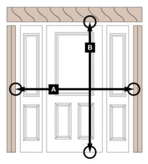
**Measurement A:** Measure from inside the face of one stud to the inside of the face of the other stud.
